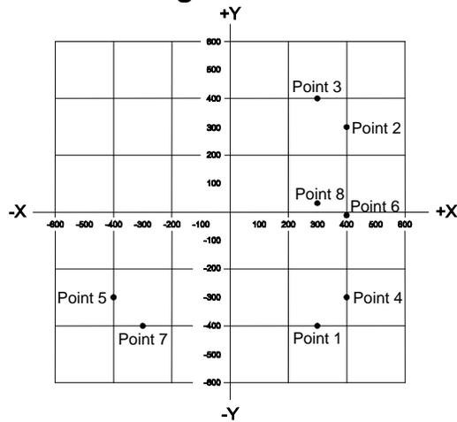
**E5C14:** Using E5-2, which point represents the impedance of a circuit consisting of a 400 Ω resistor in series with a 38-pF capacitor at 14 MHz? (p.4-23)
