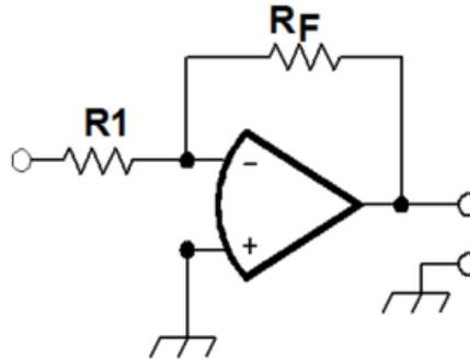
**E7G07:** What magnitude of voltage gain can be expected from the circuit in Figure E7-4 when R1 is 10 ohms and RF is 470 ohms? (p. 6-9)
